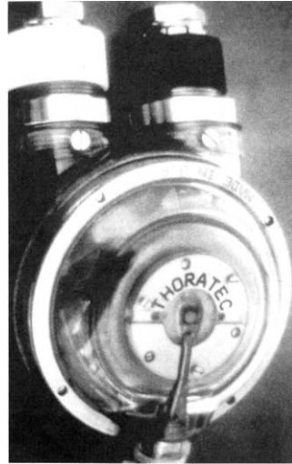
Fig. 2. Thoratec VAS extracorporeal pneumatic blood pump. (From Pagani FD, Aaronson KD. Mechanical circulatory support. In: Greenfield LJ, editor. Surgery: scientific principles and practice. 3rd edition. Philadelphia: Lippincott Williams & Wilkins; 2001. p. 1515; with permission.)
