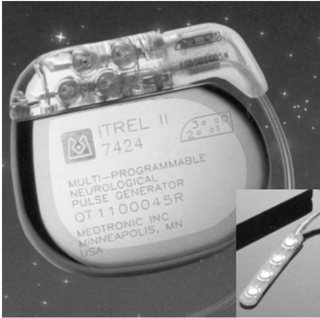
Fig. 4. The internal pulse generator used in the two pilot horses with the four-point bipolar electrode (inset) to which the first cervical nerve was attached.
