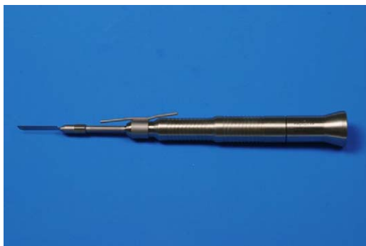
Fig. 5. Prototype of a reciprocal saw presenting an elongated but thinner shaft (Medicon Company, Tübingen, Germany).
